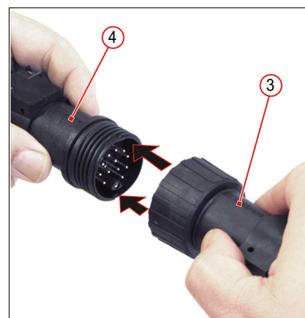
Fig. 25: Connect plug (3) and receptacle (4) in such a way that grooves and guideways slide into each other easily
